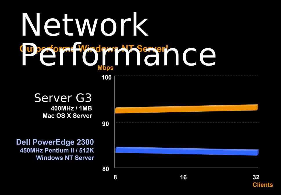
NetBench Sequential Read test of network throughput from 8, 16 & 32 Mac clients in Megabits per second (Mbps) on 100Base-T Ethernet
