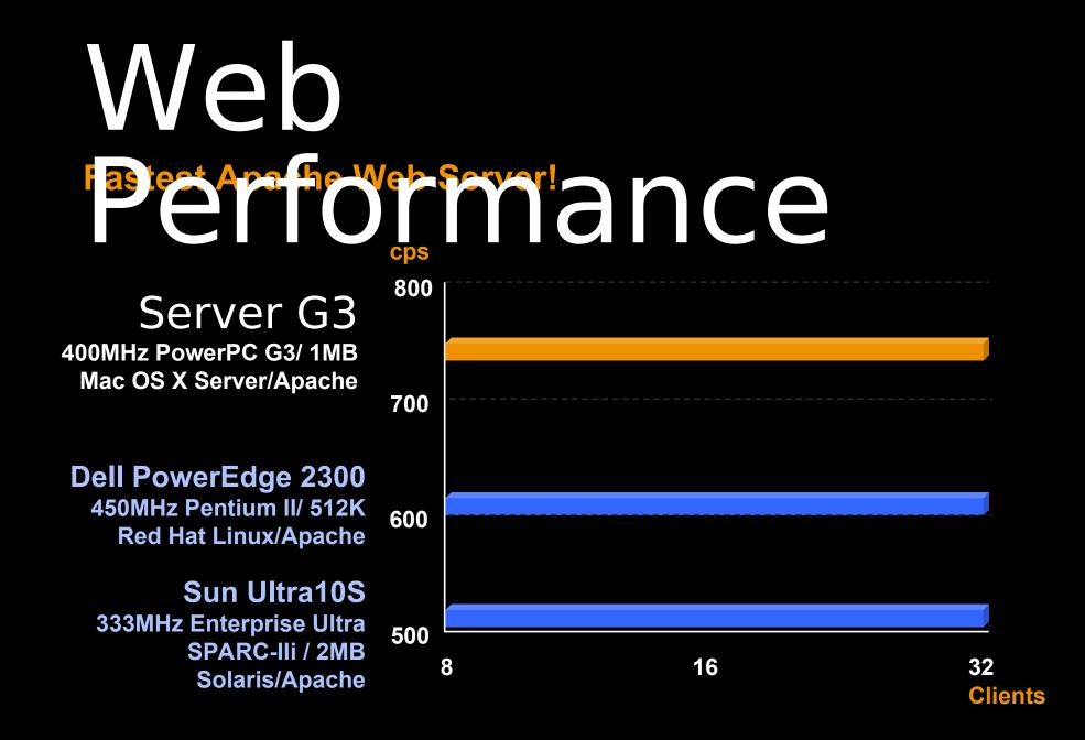
WebBench static HTML throughput from 8, 16 & 32 PC clients in connections per second (cps) on 100Base-T Ethernet
